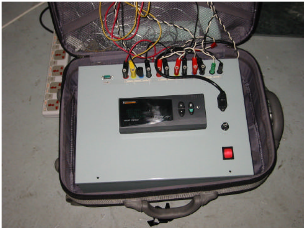
Photo#2 - Measuring Equipment (CM4000)
